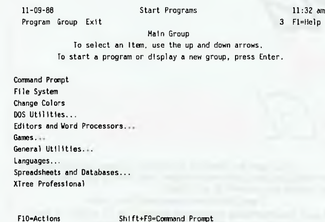
Figure 1. The initial screen (called the Main Group) can invoke up to 16 other menus, which are called groups in IBM terminology and are named by the user. Selections may be made with mouse or keyboard.
