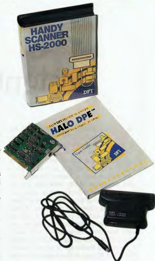
Figure 3. The Handy Scanner HS-2000 comes neatly packaged – the plastic box contains the handpiece and short slot drive card along with the single software disk and manual. The box also contains three other disks which carry the Halo DPE software and extensive manuals. The card uses a miniature DIN plug to connect a light cable to the scanner.
